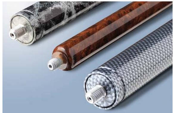
The decors are produced in the so-called dip-print process. In this process, wafer thin films are applied to the stainless steel body with pressurised water and the result is completely free of bubbles. A heavy-duty clear varnish reliably protects the surfaces against mechanical loads.
