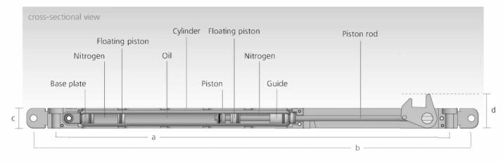
In 2015, HAHN Gasfedern presented a new product group for a smooth dampening and closing of sliding doors and other applications involving linear moved masses of ca. 40–400 kg.
